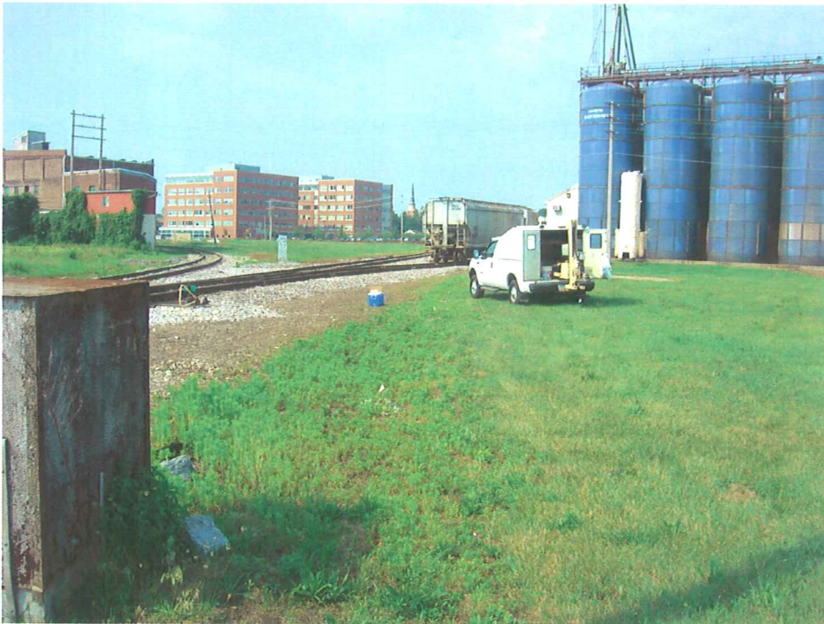
Soil sampling with a geoprobe.
